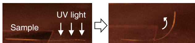
Figure 4. Photographs of P451 fiber exhibiting bending behavior in response to UV light (365 nm, 30 mW cm -2 ). White dash lines indicate edges of the fiber.
